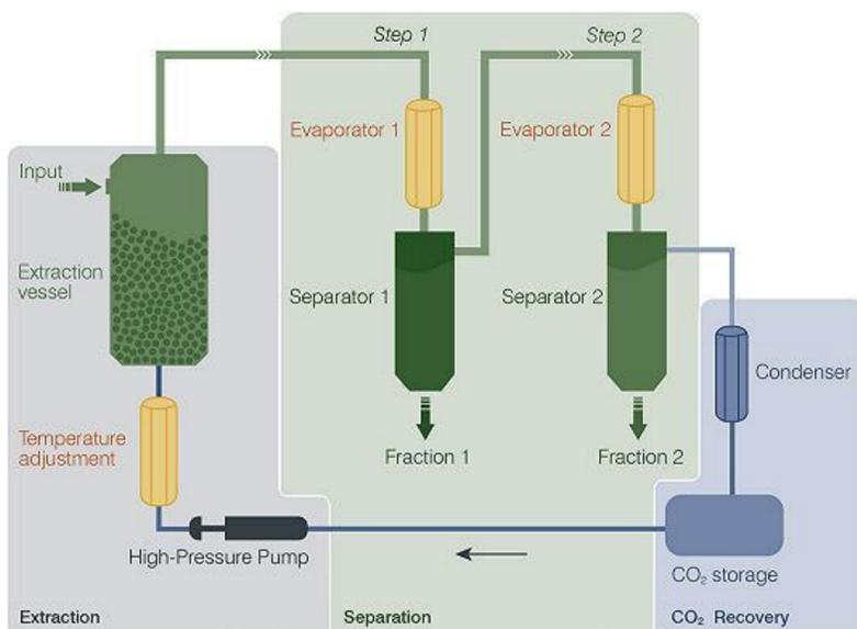
Fig. 1: Technical chart of a CO<sub>2</sub> extraction plant for calendula
